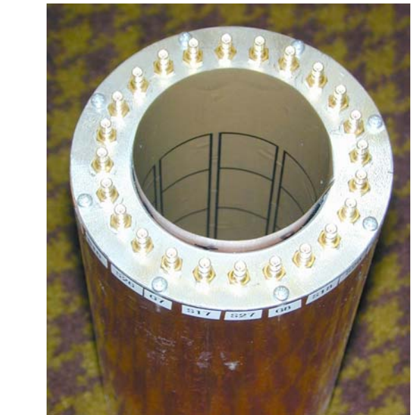
Figure 3. Photograph of sensor showing internal electrodes and connectors
